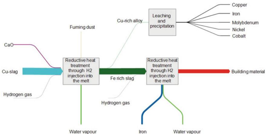
Fig. 2 Sankey diagram for the valorisation of copper slag
