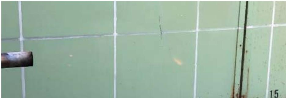
**FIGURE 1: AN ALMOST INVISIBLE HYDROGEN FLAME BURNING IN AIR**
