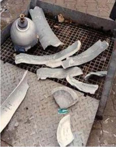
**FIGURE 3: FRAGMENTS OF A HYDROGEN CYLINDER THAT RUPTURED AFTER THE INGRESS OF OXYGEN INTO THE HIGH-PRESSURE HYDROGEN CAUSED AN EXPLOSION**
