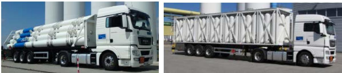
FIGURE 5: A 200 BAR HYDROGEN TUBE TRAILER AND A HIGH PRESSURE 500 BAR COMPOSITE TUBE TRAILER
